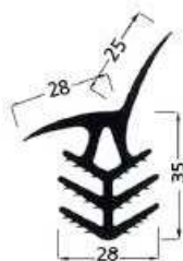
FAE 15/3035 (for corner joints) Material: MIGUFLEX Joint width: 20 mm
