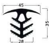
FA 15/4535 Material: MIGUFLEX Joint width: 20 mm
